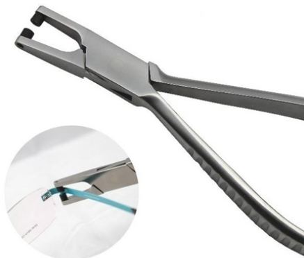
Hinge Setting or Angling Pliers AI-01-108 For hinges setting. Firm holding of joints during adjustments. With two concave indentations. Length: approx. 140 mm Weight: approx. 107.5 g
