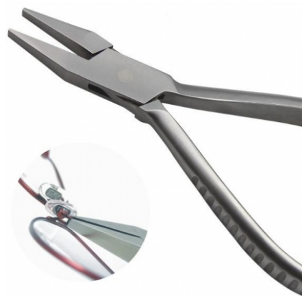
Flat Nose Pliers 4.5mm AI-01-127 Flat milled jaws with 4.5mm width for better hold. Used for general purposes, particularly useful for adjust of pad arms & holding temples on thin metal frames. Length: approx. 150 mm Jaws Width: 4.5 mm x 1.2mmH Weight: approx. 115.5 g
